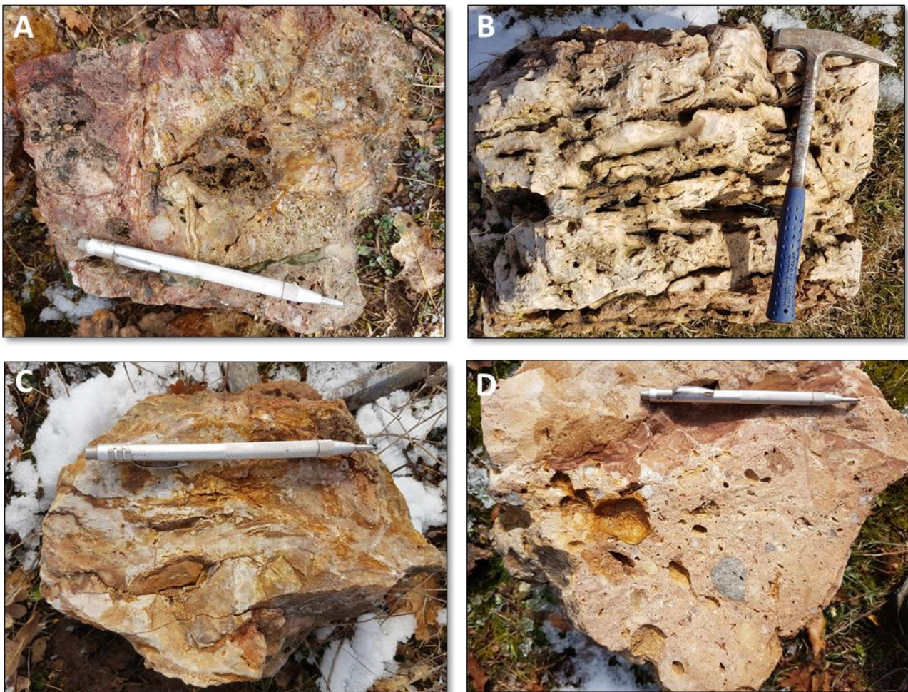
Figure 3: Selection of rocks outcropping at Makedontsi. A. Low sulfidation epithermal (LSE) stockwork and silicification. B. Epithermal quartz banded vein. C. Composite LSE vein and silicification with abundant iron oxides after pyrite. D. Silicified polymictic breccia-conglomerate.
