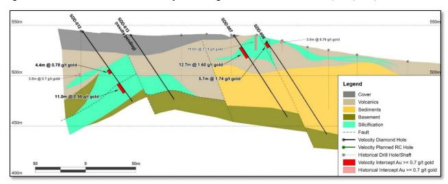
Figure 3: Cross Section at Sedefche Gold Project showing results for drill holes ODD-06, -007, -012 and -013.
