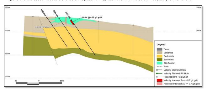
Figure 4: Cross Section at Sedefche Gold Project showing results for drill holes ODD-08, -009 and -010.
