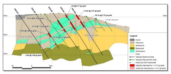
Figure 2: Cross Section at Sedefche Gold Project showing results for drill holes ODD-01, -002, -003, -004 and -005.
