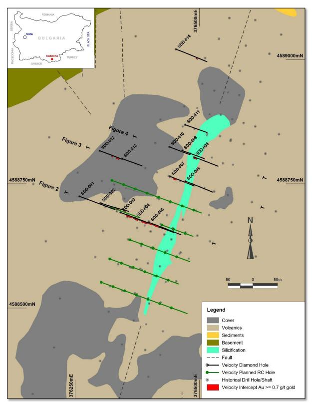
Figure 1: Map of the Sedefche Gold Project, showing the drill traces of completed and planned drilling. The drill hole locations are displayed on a geological map of the deposit including positions of previous drill collars
