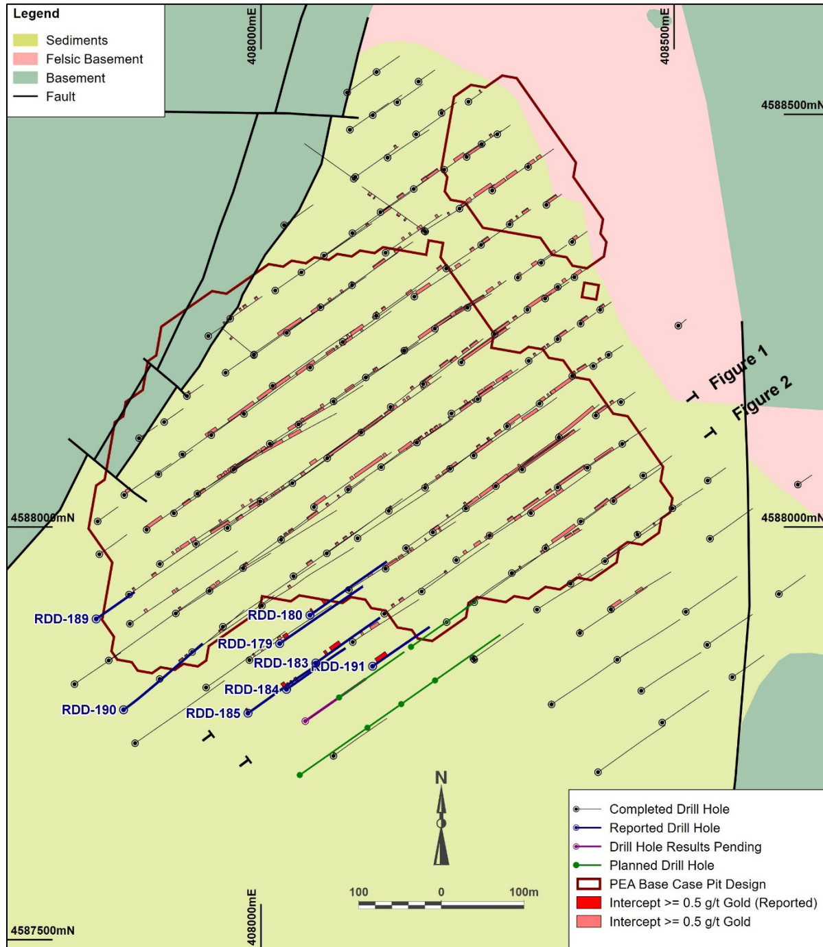
Figure 3: Mapping showing location of Rozino drill holes completed, planned drill holes and the PEA design pit limits.
