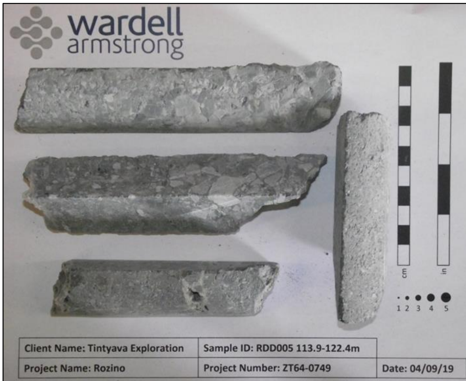
Figure 13-7: Sulphide Master Composite, RDD005, 113.9-122.4 m interval Source: WAI, 2019
