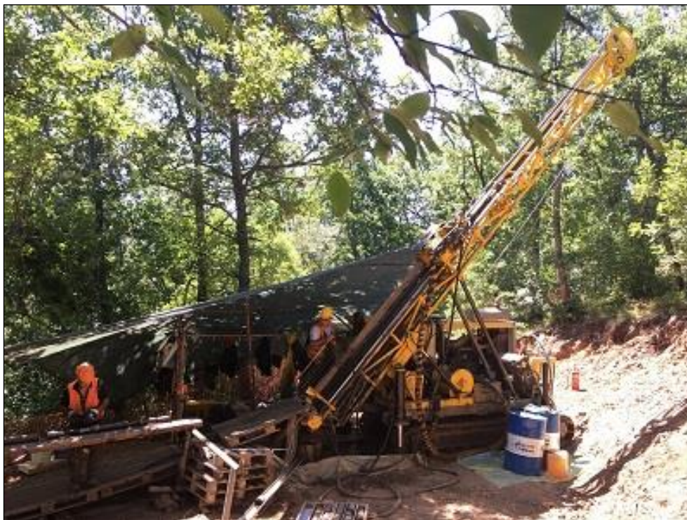
Figure 10-3: Velocity diamond drilling – drill site detail Source: Velocity, 2020
