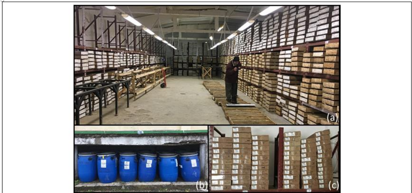
(a) Logging and core storage area, (b) Coarse reject storage in sealed plastic drums, (c) Pulp storage area
