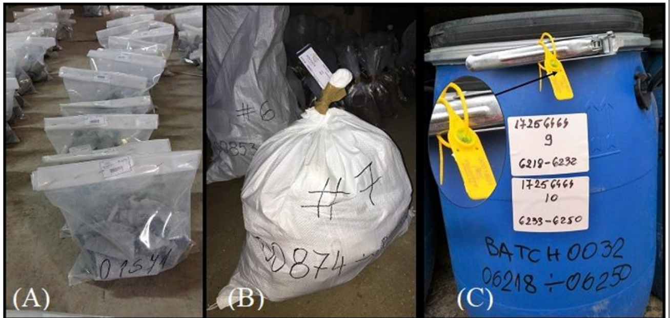
(A) Individual sample bags with sample tags (B) Polywoven bag labelled with sample sequence, (C) Plastic drum with sample and batch sequence and plastic tag seal
