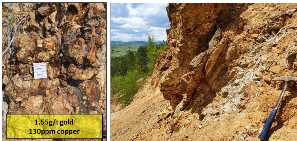
Plate 1. Outcropping QSP-altered andesitic volcanic rock sampled by Velocity, grading 1.55 g/t gold and 130ppm copper (left), and altered andesite fragmental & andesite porphyry with disseminated chalcopyrite (right).
