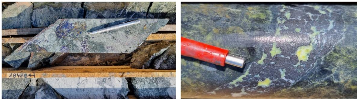
Figure 2. Skarn mineralisation with semi-massive bornite - covellite - chalcopyrite (left) and magnetite +/- chalcopyrite (right) from drill holes IDD-001 and IDD-003 respectively, Igljka Skarn.
