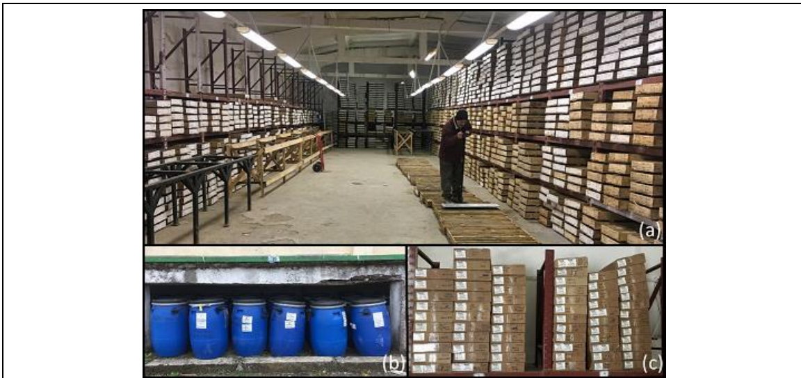
Photographs courtesy Velocity. (a) Logging and core storage area, (b) Coarse reject storage in sealed plastic drums, (c) Pulp storage area
