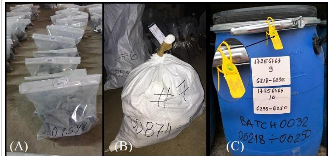
Photographs courtesy Velocity. (a) Individual sample bags with sample tags (b) Polywoven bag labelled with sample sequence, (c) Plastic drum with sample and batch sequence and plastic tag seal
