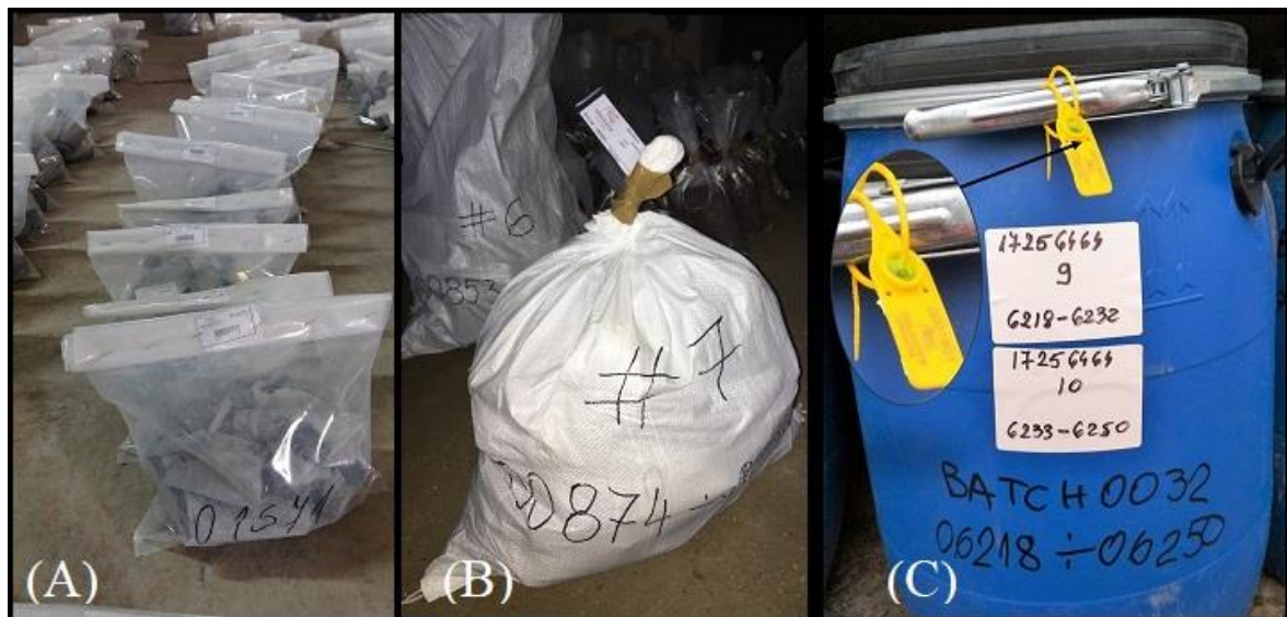
Figure 14: Velocity's Ivaylovgrad core storage facility and sample packaging: (a) individual sample bags with sample tags; (b) polywoven bag labelled with sample sequence; (c) plastic drum with sample and batch sequence and plastic tag seal
