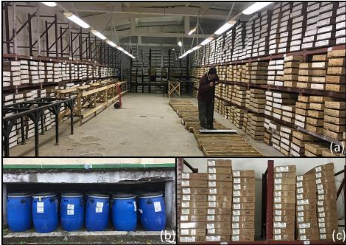
Figure 13: Velocity's Ivaylovgrad core storage facility and sample packaging: (a) logging and core storage area; (b) coarse reject storage in sealed plastic drums; (c) pulp storage area
