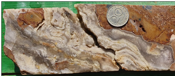
Colloform banding of silica at the Makedontsi deposit, typical of low sulphidation epithermal gold system
